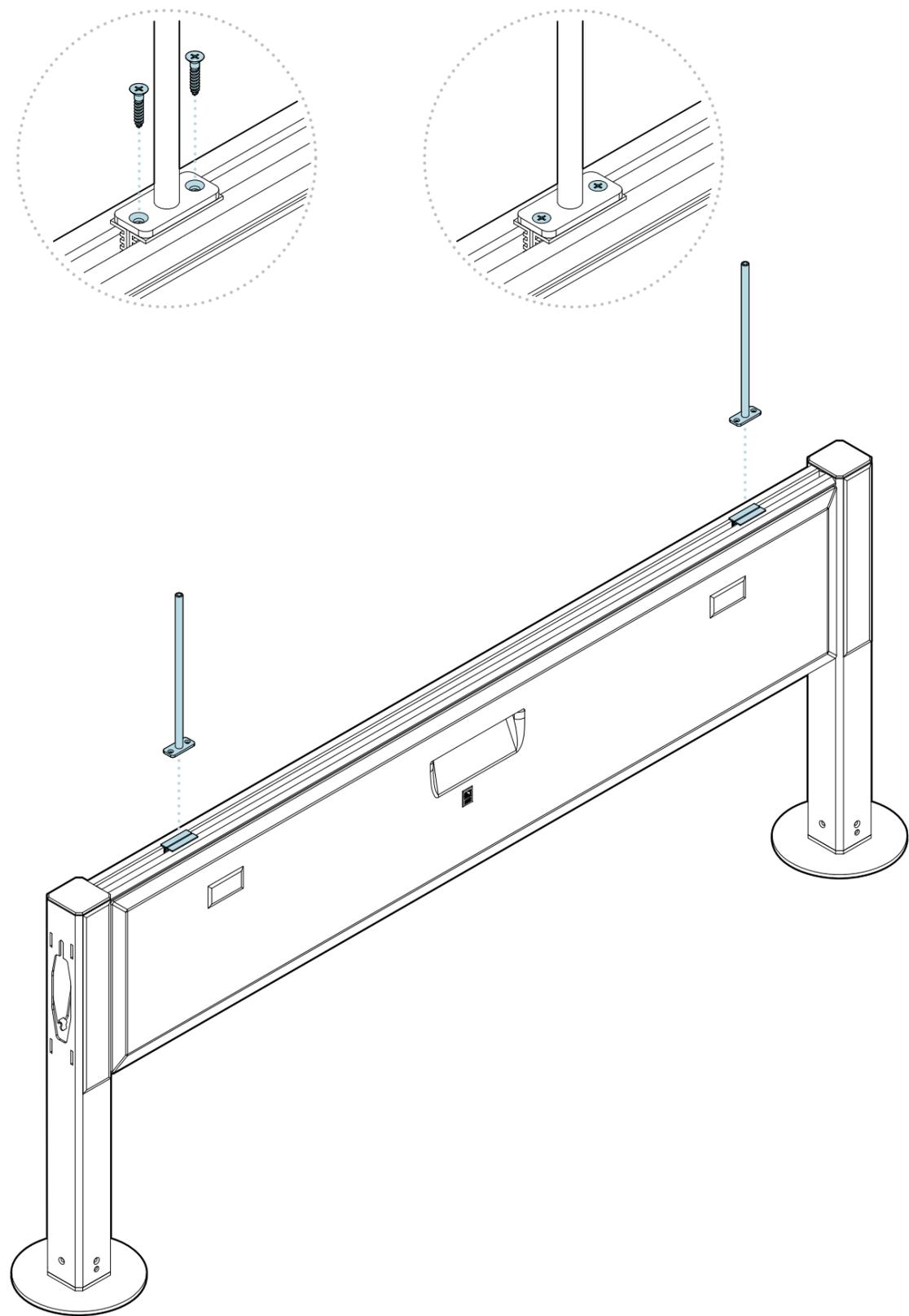
Align one T-bracket with a privacy panel adapter and lower in place. Using a Phillips head screwdriver and 2 of the provided screws, attach the bracket to the adapter. Repeat with the second T-bracket, adapter, and remaining screws. **NOTE: Ensure the T-brackets are vertical and perpendicular to the Beam. If they are not, loosen the screws and adjust as needed.**
