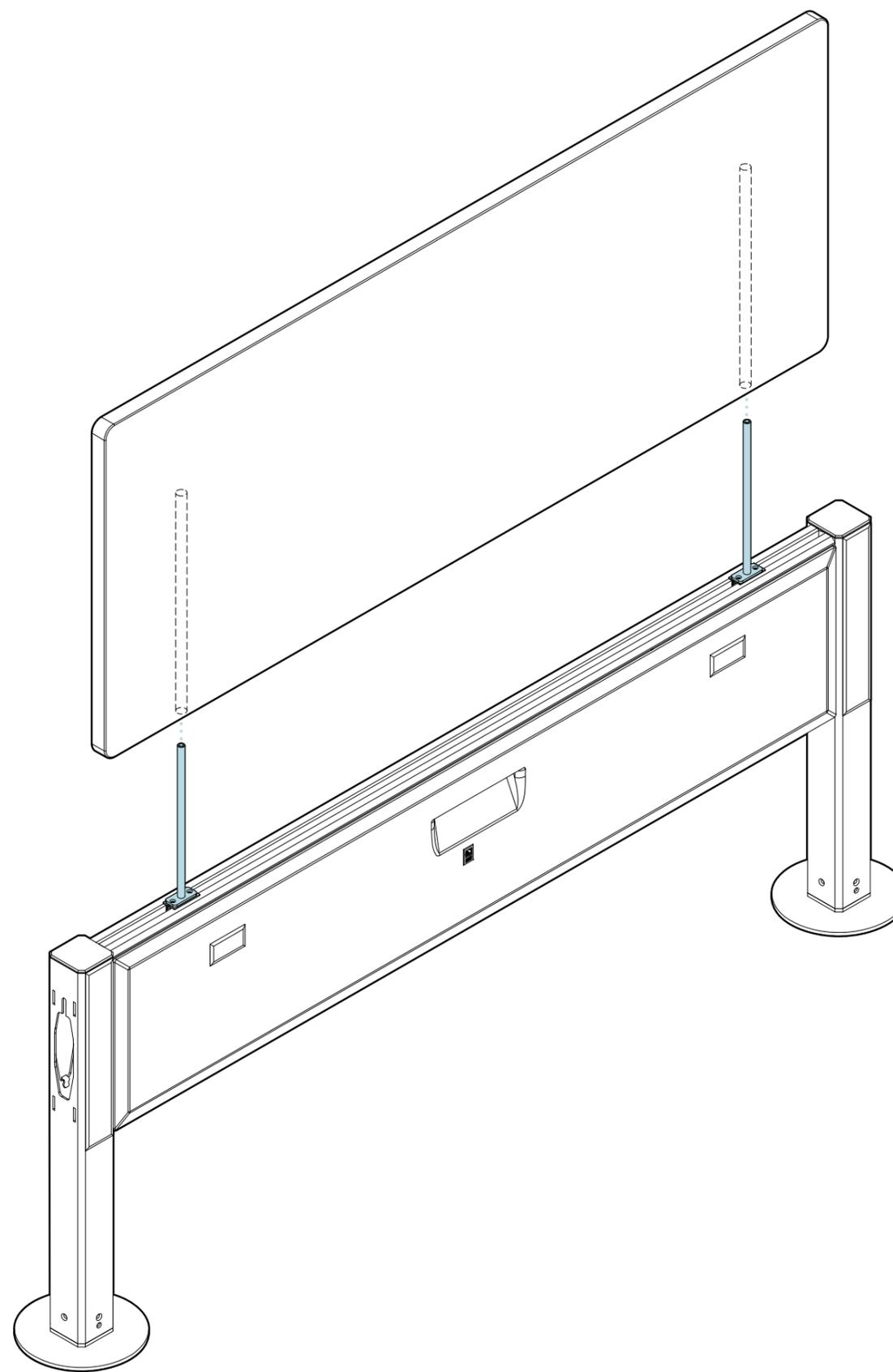
Position the panel with the predrilled holes facing down and aligned with the t-brackets, then lower the panel onto the t-brackets.
